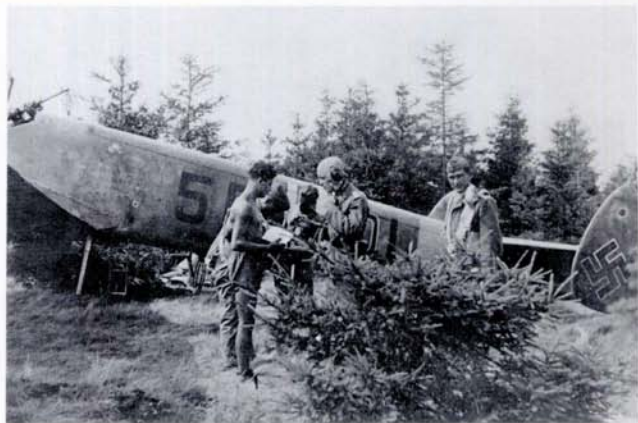
ABOVE: 5D+OL, a reconnaissance Bf 110 E-3 of 3./Aufkl. Gr. 31, forms a backdrop to aircrew activity. The yellow Russian Front theatre band can be seen on the rear fuselage. The fin is heavily mottled, in contrast to the area ahead of the unit code on the fuselage.
