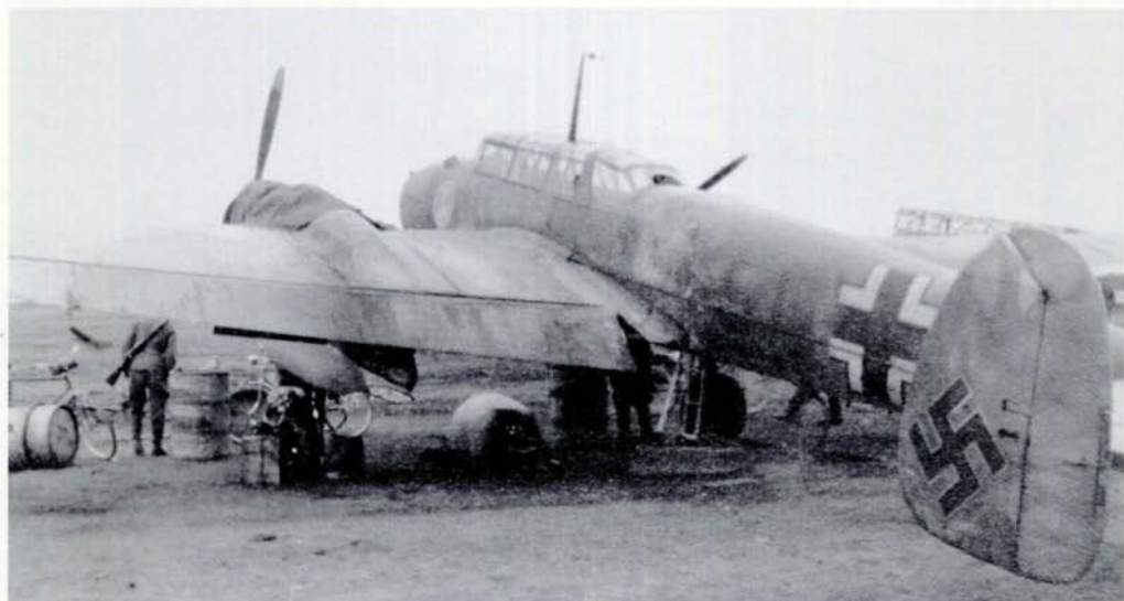
BELOW: Bf 110 C-2, KD+TB, W. Nr. 2132, that has previously been deployed to towing duties. Seen here with NJG Schule 1, it carries the number '10' on the rear fuselage and an unidentified emblem on the nose. The towing features, of rear view mirrors ahead of the pilots' windscreen, enlarged radiators (required due to the low speed involving in towing huge transport aircraft) and shortened rear fuselage housing the pulley system. This Bf 110 retained its early-war style solid upper surface camouflage.
