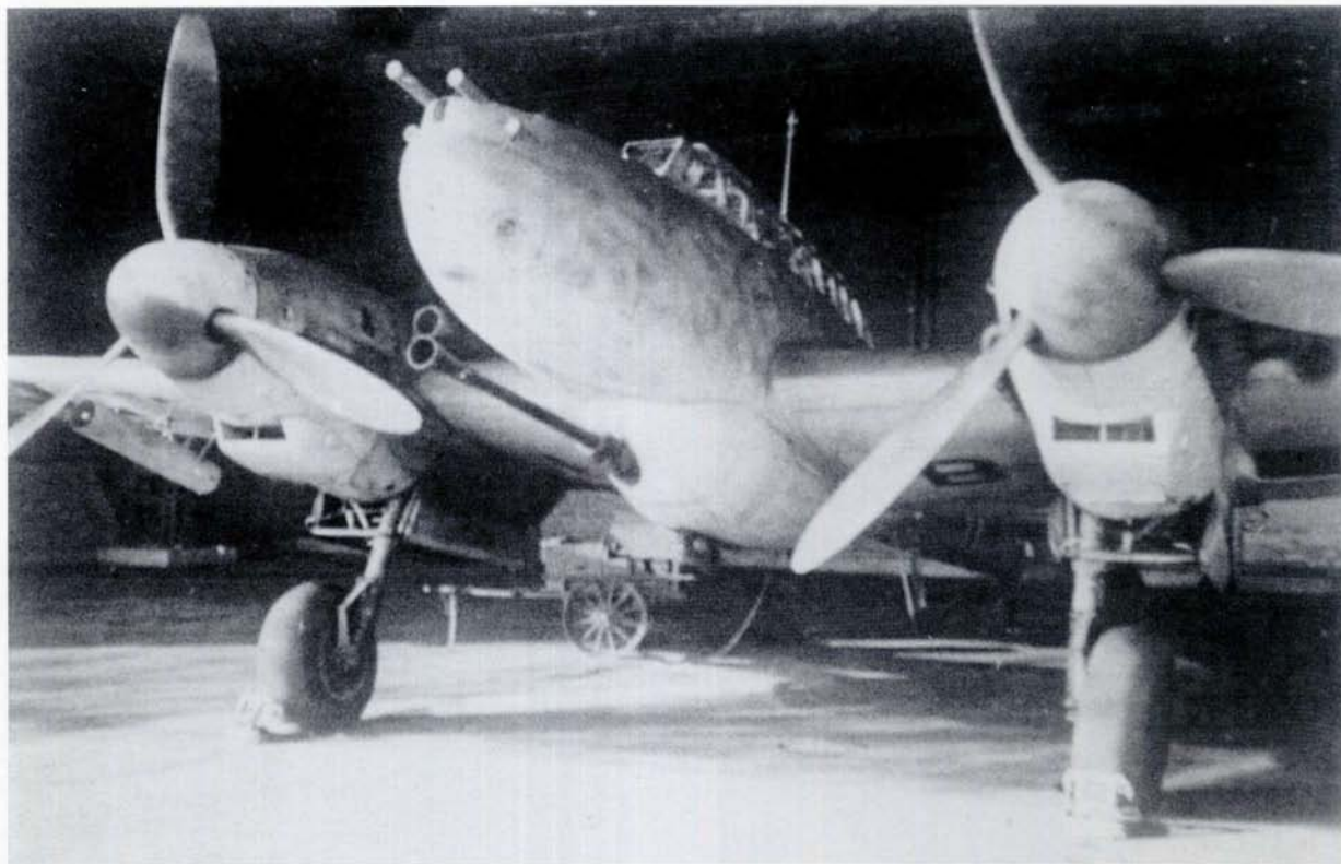
ABOVE: This Bf 110 G-2 is fitted with an unusual mix of forward-firing armament, consisting of the 3.7 cm cannon under the fuselage, four machine guns in the upper nose, and a single W. Gr. mortar tube under each wing.
