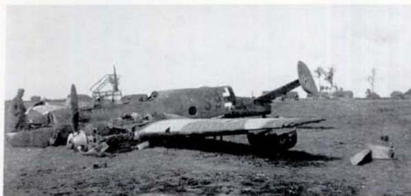
ABOVE: 2./SKG 210 Bf 110 after a heavy landing. Note the letter 'A' on the engine cowling on the ground, denoting the fitment of the DB 601 A engine. The strong contrast between the two camouflage colours on the wings would indicate the application of RLM 71 and 02.
