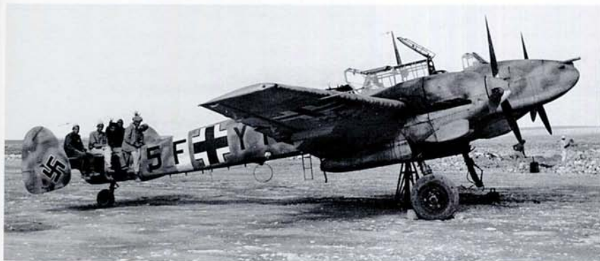
RIGHT: 5F+ZK, a Bf 110 E-3, showing the tropical filter and enlarged radiator fitted to combat the conditions of the African theatre. The emblem of 2./Aufkl. Gr. 123 remains on this Bf 110 of Aufkl. Gr. 14 also.
