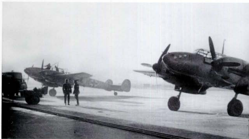
LEFT: Bf 110 D, 2N+AN, of 8./ZG 76, displaying the extended rear fuselage common to the variant. The letter 'A' appears to be black outlined in white.
