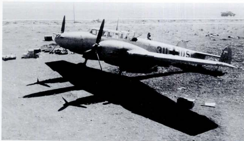
LEFT: Bf 110 E, 3U+DS, in what appears to be a single overall upper surface camouflage colour. The individual aircraft letter 'D' is in the Staffel colour of red, a reversion to the pre- and early-war colour used. It has no outline to it, having the white theatre band as a background. The spinner tip is in red also, and the port fin displays several victory bars.
