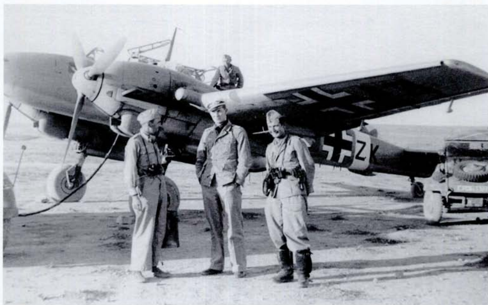
RIGHT: 5F+ZK, a Bf 110 E-3, showing the tropical filter and enlarged radiator fitted to combat the conditions of the African theatre. The emblem of 2./Aufkl. Gr. 123 remains on this Bf 110 of Aufkl. Gr. 14 also.
