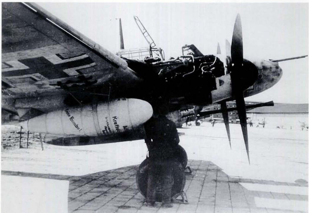
BELOW: This Bf 110 G-2 day fighter packs a powerful punch in its forward firing armament, with a 3.7 cm cannon under the fuselage and two MG 151/20 cannon in the top of the nose. Of interest is the stencilling on the supplementary fuel tank under the wing, particularly the words 'Keine Bombe!' (not a bomb!). The lower starboard wing appears to be painted yellow from the wingtip to a point just outboard of the cross.
