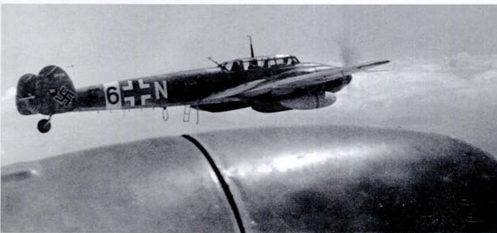
LEFT: In-flight view of an Aufkl. Gr. 122 Bf 110 E-3, with the fuselage band behind part of the fuselage code. Note the supplementary fuel tank under the wing, and the W. Nr. 2448 on the fin.
