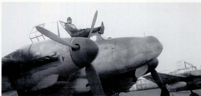
RIGHT: 1./ZG 26 Bf 110 G-2s at Bad Lippspringe in late 1943. Note that no armament is carried in the upper nose of the nearest aircraft, but a pair of MG 151/20 cannons in a ventral tray is in place under the fuselage. The Bf 110 G-2 alongside it carries a broad white fuselage band on the rear fuselage and a supplementary fuel tank under the starboard wing.
