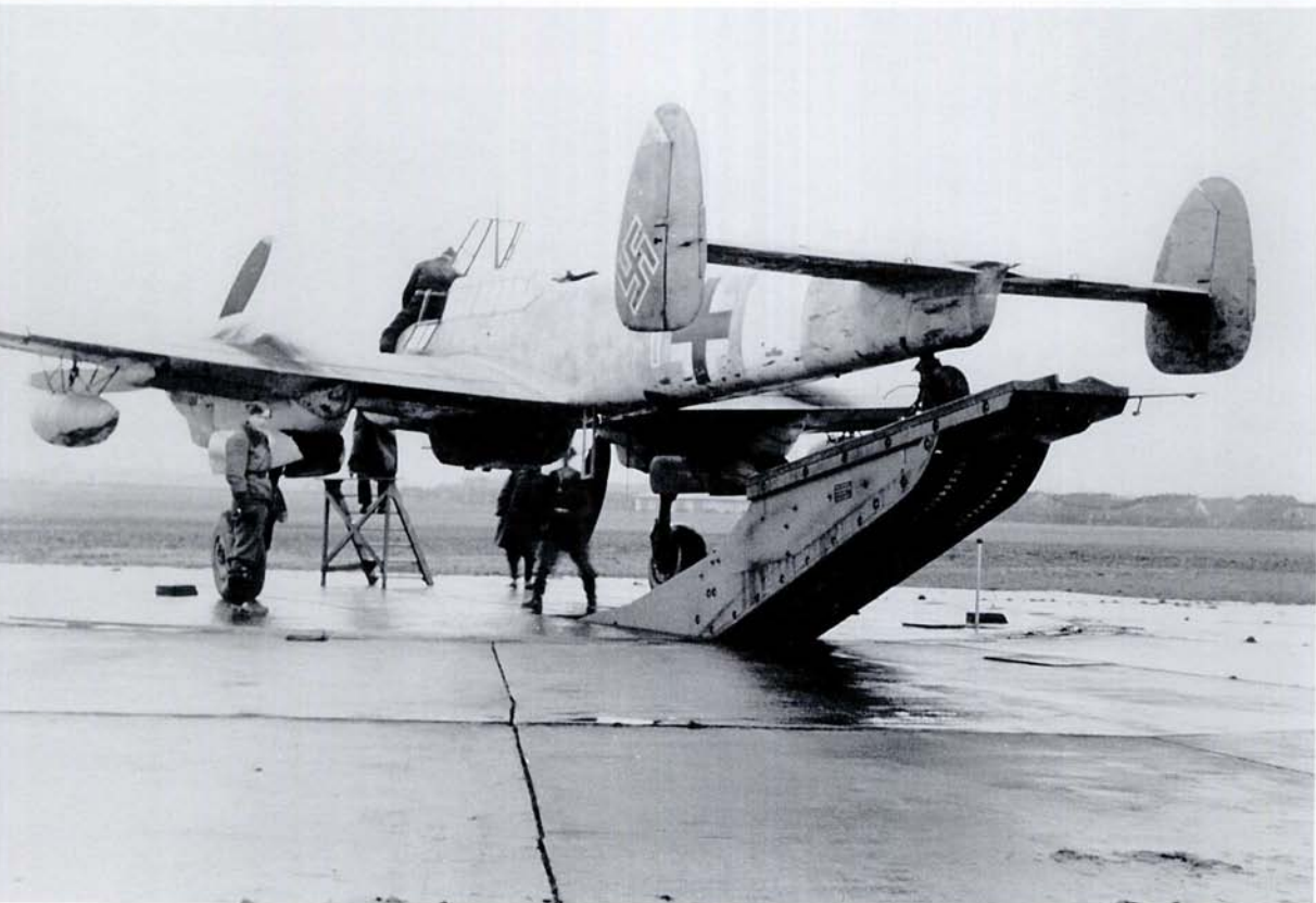
LEFT AND BELOW: Two views of a Bf 110 G-2 'Yellow 1' of an unidentified unit having its compass calibrated. Supplementary fuel tanks are fitted under the wings and the twin MG 151/20 ventral pack is fitted. A wide white band is carried on the rear fuselage, and the fuselage cross does not have any thin black outline to it.
