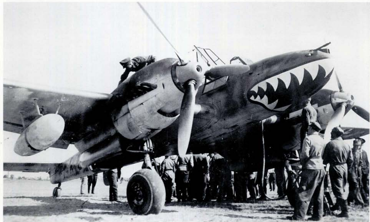
BELOW: Bf 110 E of IL/ZG 26 fitted with under-wing supplementary fuel tanks, but lacking a bomb rack.
