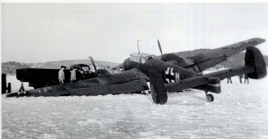
ABOVE AND RIGHT: Two views of a Bf 110 of III./ZG 76 that has suffered port undercarriage failure. Note the light area around the extended rear fuselage.
