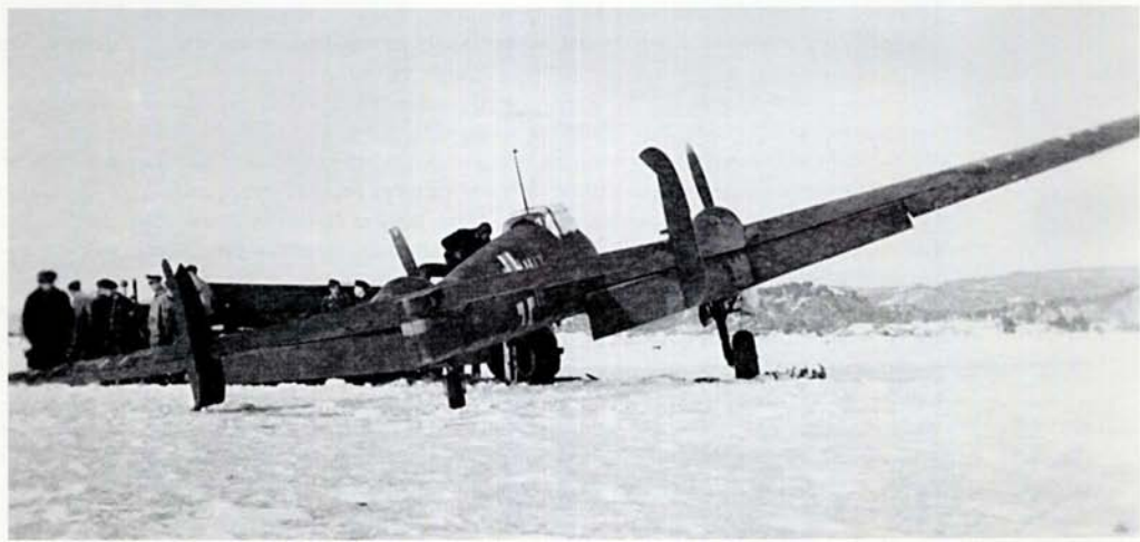
ABOVE AND RIGHT: Two views of a Bf 110 of III./ZG 76 that has suffered port undercarriage failure. Note the light area around the extended rear fuselage.
