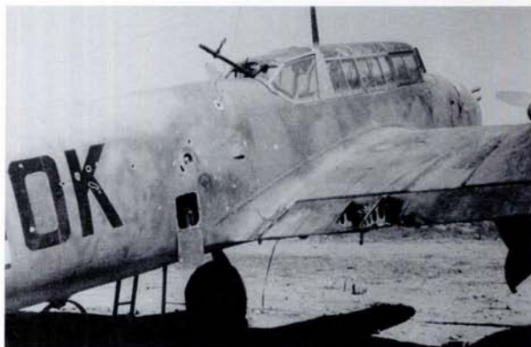
ABOVE: Bf 110 E-3, 5F+OK, of 2./Aufkl. Gr. 14 showing a two tone upper surface camouflage pattern, and damage to the fuselage and starboard flap.
