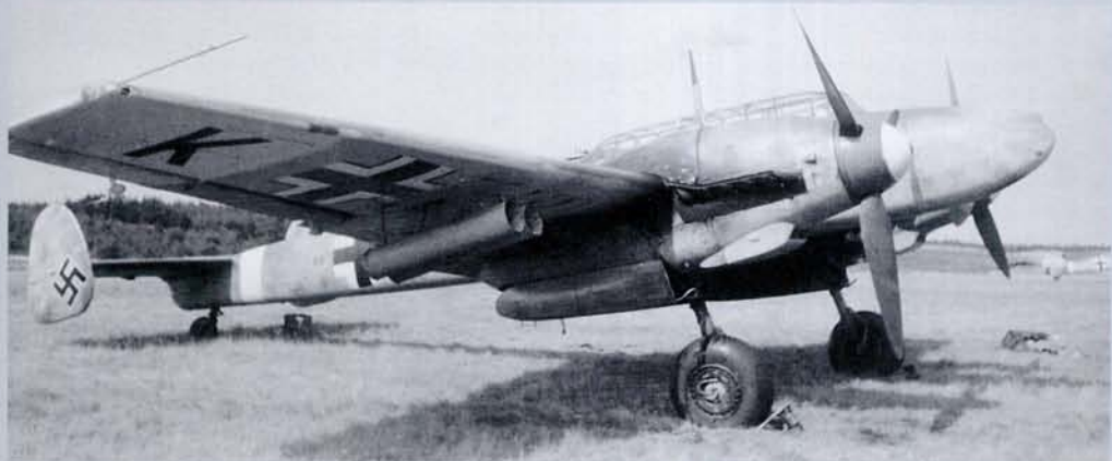
LEFT: This Bf 110 G-2 of 7/ZG 26, coded 3U+KR carries a white rear fuselage band and two mortar tubes under each wing. The underside of the starboard wingtip appears to be painted in yellow, with the individual aircraft letter, 'K', painted on it.
