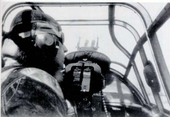
LEFT: This view of the Bordfunker's cockpit area of a ZG 1 Bf 110 G-2 shows the W. Nr. 5243 repeated twice on the panel in front of the Bordfunker. The MG 81 Z twin machine guns are shown to excellent effect, as are the twin gunsights.
