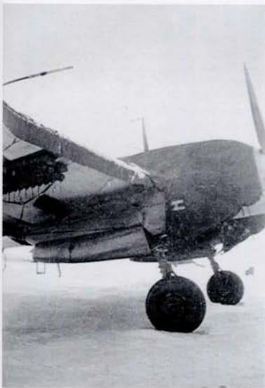
ABOVE: SD 2 bombs can be seen on the starboard bomb rack of this Bf 110 in the midst of a Russian winter.
