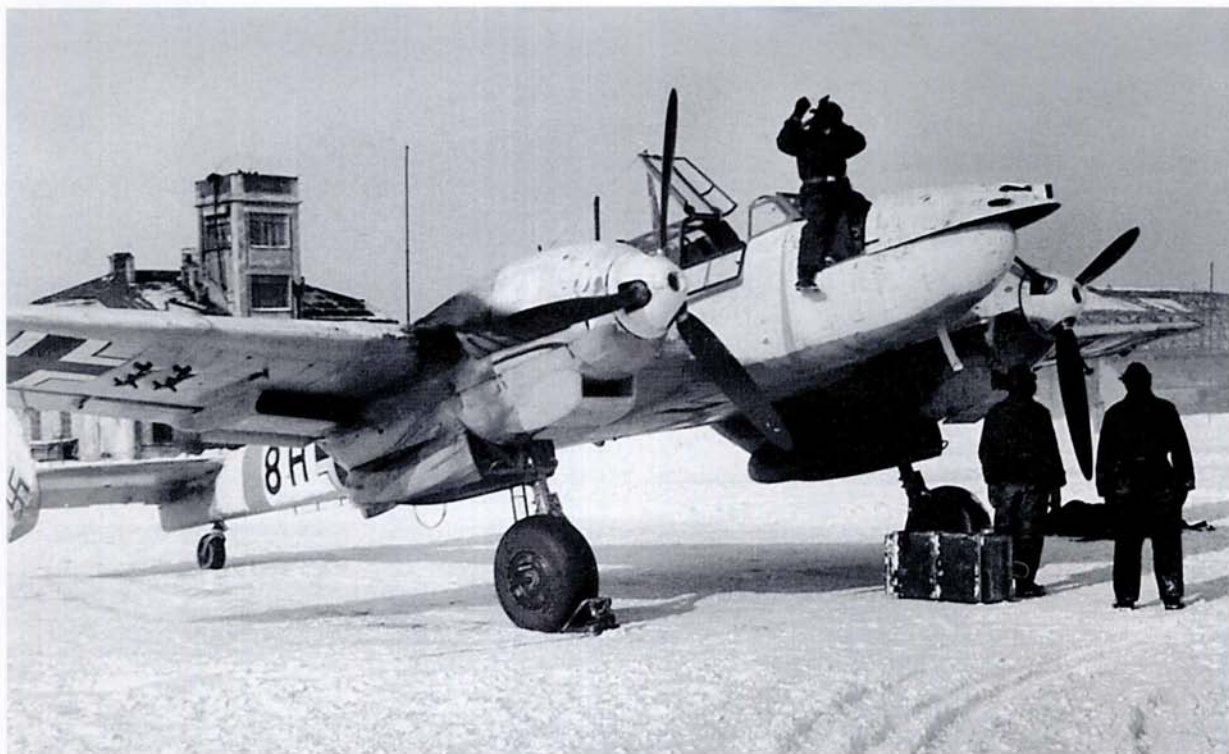
ABOVE: Bf 110 E-3 of I. Gruppe, (F)/Aufkl. Gr. 33 in the midst of the Russian winter. White winter camouflage has been applied to the aircraft, with what appears to be a fresh coat over part of the starboard engine cowlings. Although the central bomb rack is not fitted in order not to obscure the operation of the camera, bomb racks remain under the wings. The yellow Russian theatre band can be seen on the rear fuselage. An armoured windscreen is fitted, but the canopy frame has been left in its original colour, not overpainted with white.
