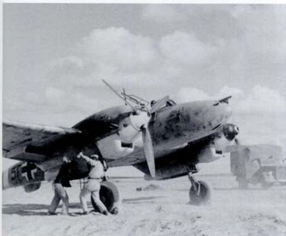
BELOW: With the port engine running, mechanics crank the starboard engine of this 2./Aufkl. Gr. 14 Bf 110 E-3. As in previous photos, this machine is fitted with tropical equipment. Two tone upper surface camouflage is carried, and the colour of the lower engine cowlings is noteworthy. Contrasting it with the white on the propeller spinners would suggest that this colour is yellow, or a fresh application of the light blue undersurface colour.
