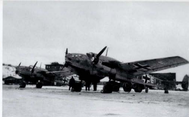
ABOVE LEFT: The three wasps emblem of III./ZG 76 can be seen on this Bf 110 E. Note also the bomb rack under the fuselage.
