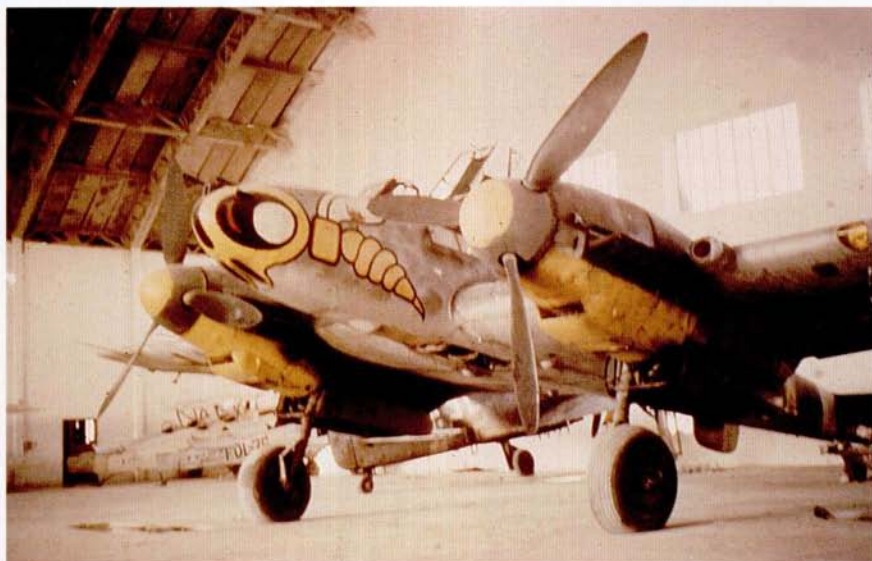
LEFT: Bf 110 G-2 of II./ZG 1 seen in Italy in 1943. Note the yellow tips to the spinners and the yellow lower engine cowlings. An armoured windscreen is fitted.
