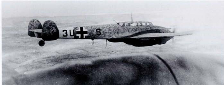
Two views of Bf 110 C-6 3U+XS of 8./ZG 26 in the desert. 3U+XS was one of three Bf 110 C-6s originally on charge with Erpr. Gr. 210 that went through repair facilities and were re-issued to ZG 26. The top surface camouflage is a single base colour with a tight 'scribble' pattern applied over it. Regarding the use of the C-6 by ZG 26 in the desert, an RAF Intelligence report stated the following: "...After a low level attack on 15.11.41 on the aerodrome at Giarabub by Me 110s, a 30 mm armour-piercing shell was found in the LFF set of a Blenheim IV damaged on the ground..."
