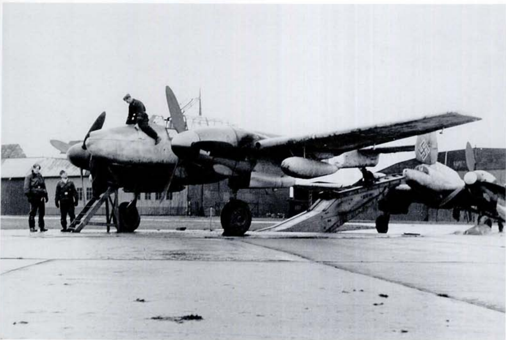
LEFT AND BELOW: Two views of a Bf 110 G-2 'Yellow 1' of an unidentified unit having its compass calibrated. Supplementary fuel tanks are fitted under the wings and the twin MG 151/20 ventral pack is fitted. A wide white band is carried on the rear fuselage, and the fuselage cross does not have any thin black outline to it.
