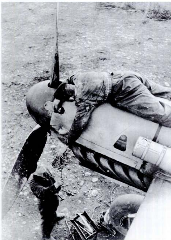
LEFT: Maintenance taking place on the port engine of a Bf 110 G-2. Note the small rectangular window on the engine cowling that allowed mechanics to check the reading on the three dials attached to the engine. Note also the fitment of a tropical filter.
