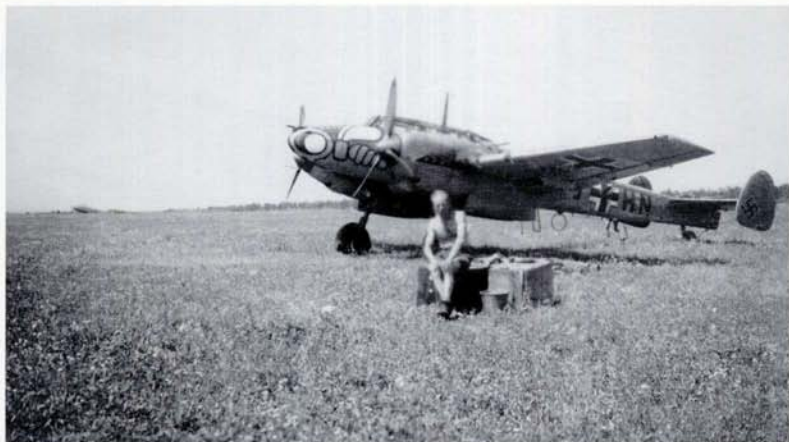
LEFT AND BELOW: Two views of S9+HN, a Bf 110 E of 5./ZG 1. Note the extended rear fuselage, and the yellow tactical marking on the lower port wingtip. An armoured windscreen is fitted, and the spinners are capped.
