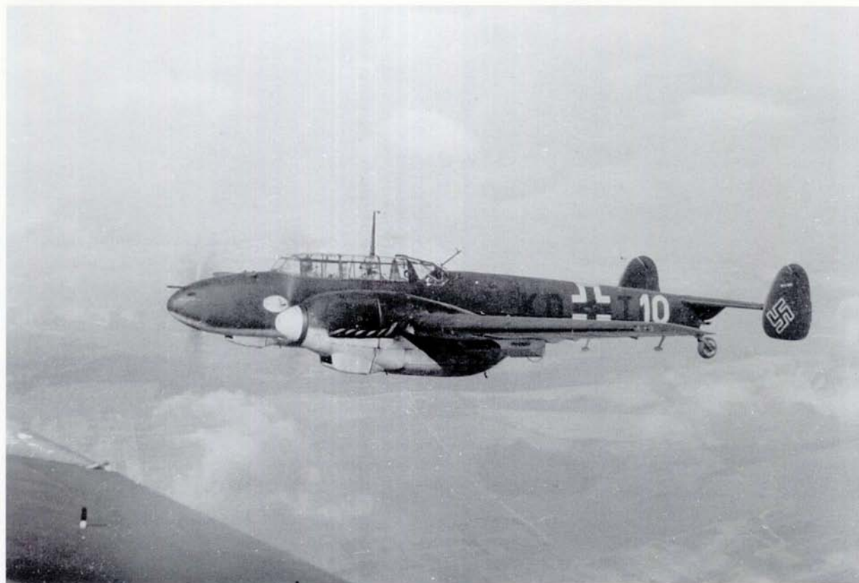
BELOW: Bf 110 C-2, KD+TB, W. Nr. 2132, that has previously been deployed to towing duties. Seen here with NJG Schule 1, it carries the number '10' on the rear fuselage and an unidentified emblem on the nose. The towing features, of rear view mirrors ahead of the pilots' windscreen, enlarged radiators (required due to the low speed involving in towing huge transport aircraft) and shortened rear fuselage housing the pulley system. This Bf 110 retained its early-war style solid upper surface camouflage.
