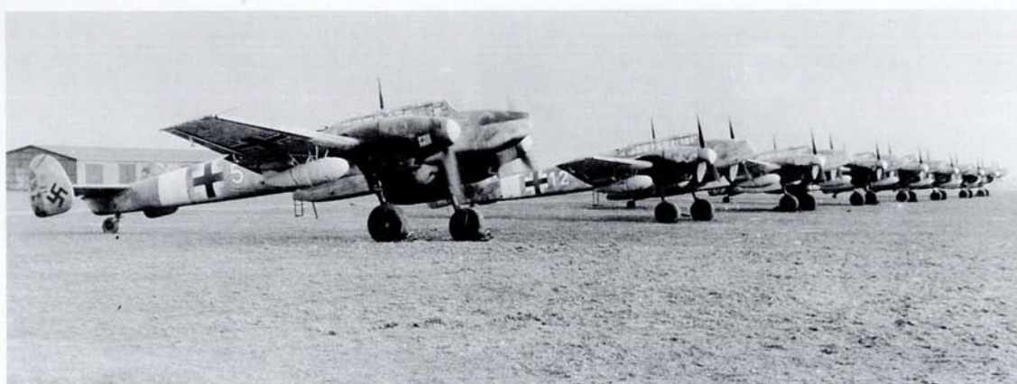
A view of I./ZG 26 Bf 110 G-2s at Bad Lippspringe in late 1943. Underwing fuel tanks are fitted to the aircraft, and 'White 5' has the MG 151/20 belly cannon pack fitted.
