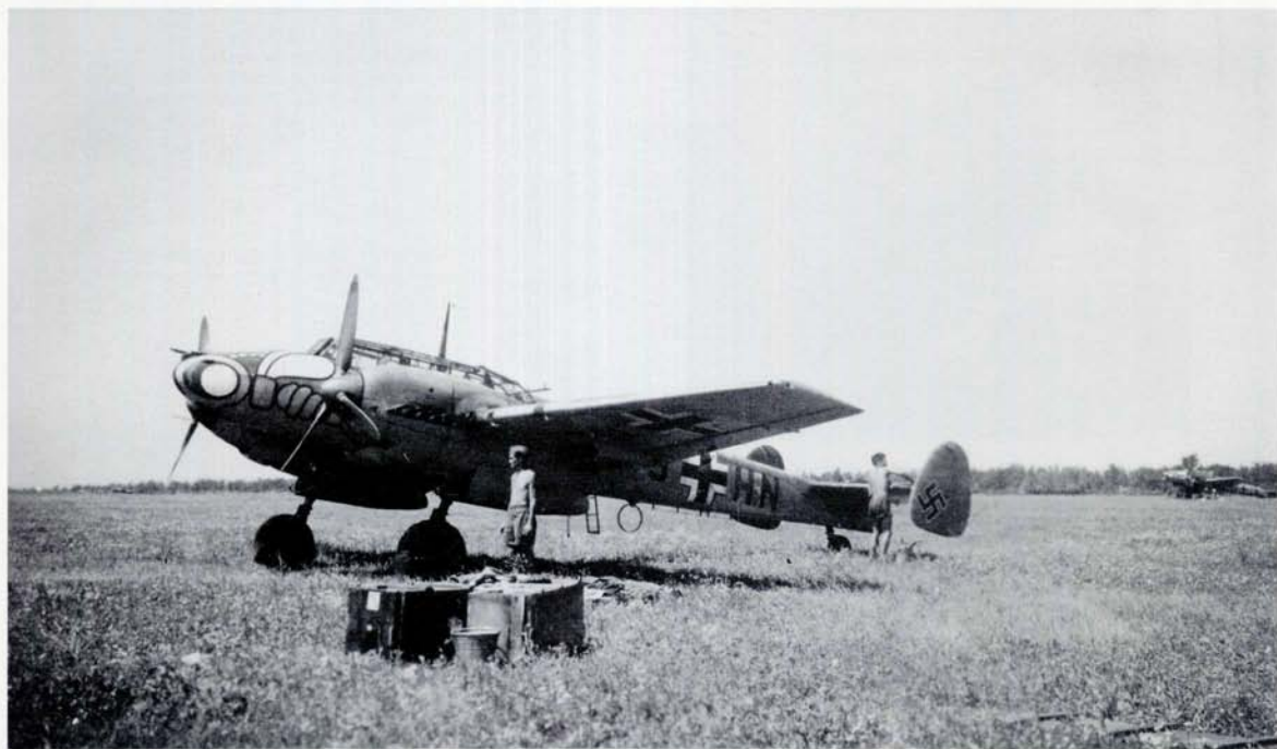
LEFT AND BELOW: Two views of S9+HN, a Bf 110 E of 5./ZG 1. Note the extended rear fuselage, and the yellow tactical marking on the lower port wingtip. An armoured windscreen is fitted, and the spinners are capped.
