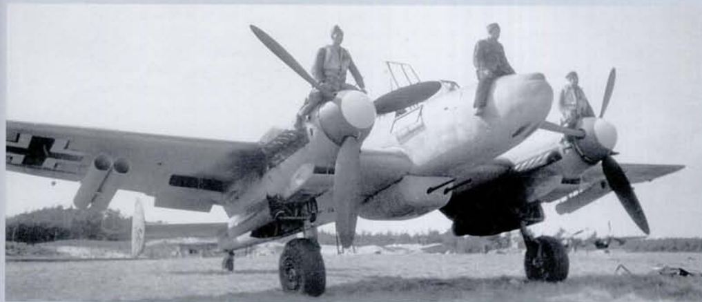
LEFT: A crew poses proudly on the engines of their Bf 110 G-2 with a mechanic on the nose. As well as the two mortar tubes under each wing, this Bf 110 G-2 has two MG 151/20 under the central fuselage. Note that the machine guns have been removed from the upper nose section.
