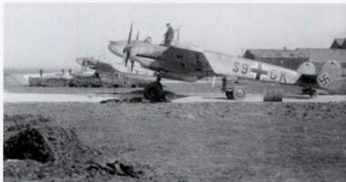
ABOVE: Bf 110 Es of 2./Erpr. Gr. 210, S9+GK, and S9+EK in the distance. Note the rectangular air inlet on the nose; a feature first introduced on the 'E' variant, and the cable running along the top of the fuselage attached to the dinghy enclosed in the extended rear fuselage. On later production batches of the 'E' the extended rear fuselage housing emergency equipment was dispensed with, the shortened rear fuselage of the 'B' and 'C' variants returning.
