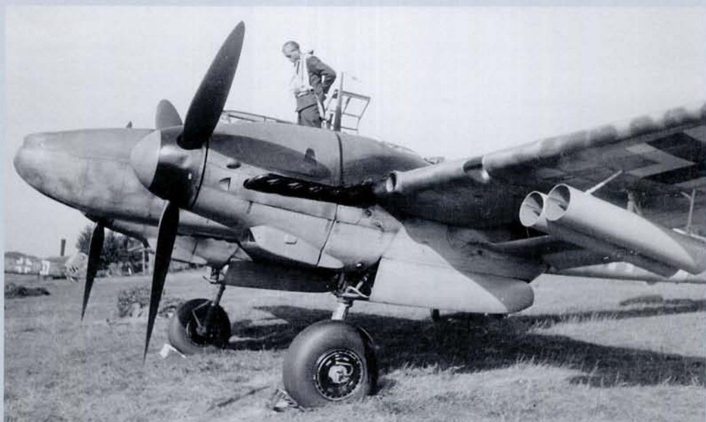
RIGHT: Bf 110 G-2 with two mortar tubes beneath each wing and a very distinctive camouflage pattern on the leading edge of the port wing.
